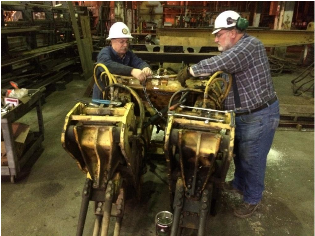
Mike H. and Frank begin work on the new-old tamper's work-head.
